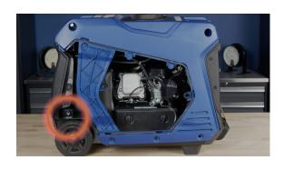
**16.** To remove the panel first, pull it out from under the black muffler at the back of the generator.
