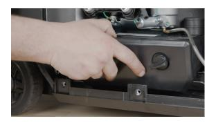
**25.** Unlock the lower air cleaner cover and remove it. Then remove the foam filter and the metal plate inside.
