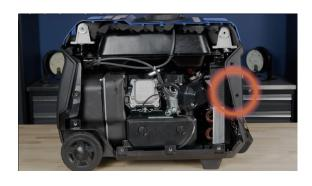
**17.** Next, pull the panel out from underneath the control panel frame, and pull the panel free.
