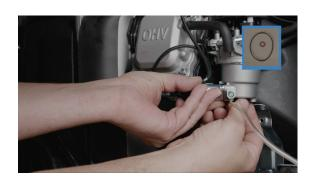
**32.** If they are damaged, replace the o-ring where the bowl meets the carburetor, and the bolt seal on the bottom of the carburetor, with the parts supplied in the kit. Re-bolt the bowl onto the bottom of the carburetor.
