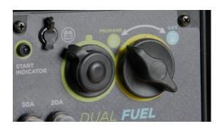
**6.** Next, turn the fuel switch to off or propane on the dual fuel model.
