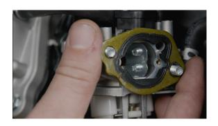
28. Remove the gasket on the front of the carburetor.
