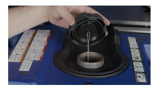
**5.** Next, you will use the carburetor drain hose to drain the gas out of the fuel tank.
