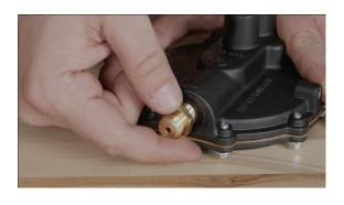
**34.** This last step is for Dual Fuel generator owners. Replace the brass jet on your propane regulator with the appropriate model that came with your kit.
