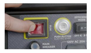
7. Flip the red switch to the "stop" position.
