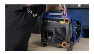
**13.** Remove the rubber plug and the 3 screws on the back left corner of the generator.
