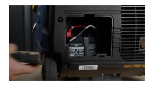
**8.** Start the disassembly by removing the battery cover and disconnecting the battery.
