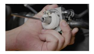
**30.** After the carburetor is removed, use the small flathead screwdriver to carefully remove the jet. Make sure the main nozzle stays in the carburetor. If it falls out, replace it in the correct orientation.
