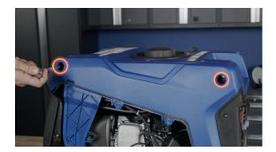
**15.** Finally, remove the 2 bolts on the left hand side, that attach to the handles.
