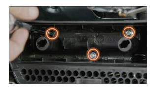
**26.** Remove the 3 bolts inside the lower air cleaner and remove the air cleaner.
