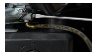
**19.** Loosen the carburetor drain screw and empty the gasoline out of the float bowl. When the float bowl is empty, re-tighten the drain screw
