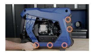
**11.** Now we're going to remove the left generator cover, start by removing the 3 bolts at the bottom of the cover, and the 2 side screws on the control panel frame.
