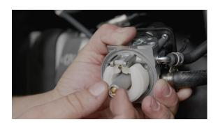
**31.** Install the new jet into the carburetor. As mentioned earlier, make sure you're installing the correct jet for your model of generator and for the altitude. After you install the new jet, don't throw away the old one.
