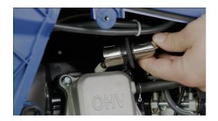
10. Remove the spark plug boot from the spark plug.
