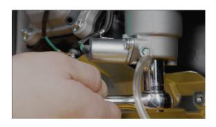
**27.** Remove the bolt from the bottom of the carburetor float bowl. There may be some leftover fuel in the carburetor so have a rag handy to clean any spills.
