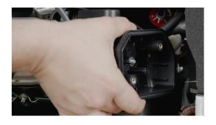
**24.** Now pull the air cleaner off the carburetor and remove it.
