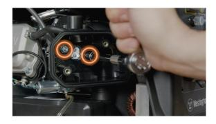
23. Remove the 2 bolts inside the air cleaner.
