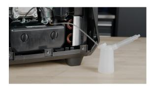
**18.** Pull the clear plastic tube from the bottom of the carburetor, and place the end of it in a gasoline safe container.
