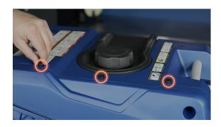
12. Remove the 3 rubber plugs, and 3 screws on the top.
