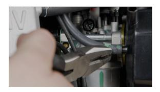
**20.** Now we're going to remove the air cleaner housing, start by remove the crankcase breather tube, and vapor tube.
