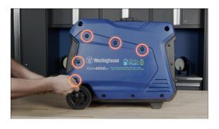
**9.** Now remove the 1 bolt and 4 screws on the left side engine service panel, and remove the panel. Keep track of the screws and bolts as you disassemble the generator housing.
