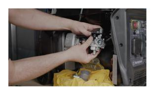
**29.** And remove the carburetor from the engine. It's a tight fit, so you may have to slowly rock the carburetor back and forth on the 2 studs that hold it to the engine
