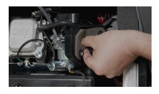
**22.** Remove the air cleaner cover and the foam filter inside.
