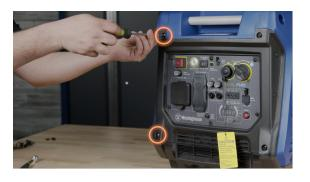
**14.** Remove the 2 screws on the left hand side of the control panel frame.
