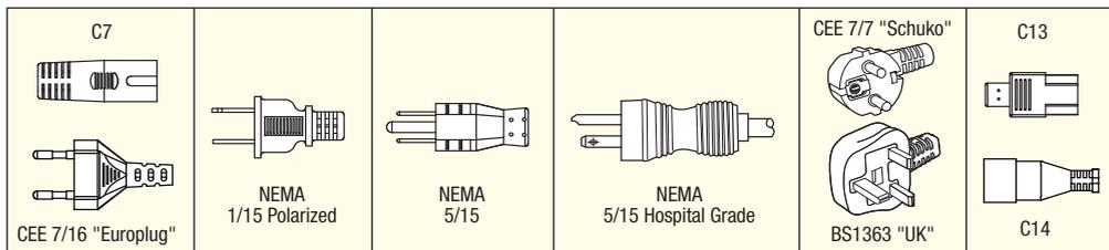
**Switching Power Supplies, Power Cords, PoE Power Supplies and Lighter Power Adapters**
