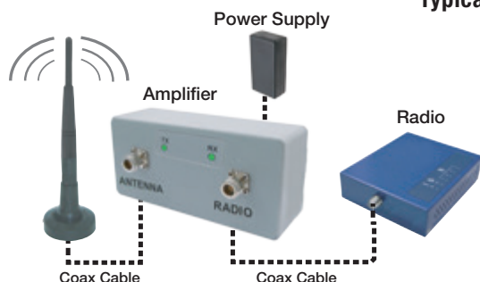
Indoor Amplifier Connection Diagram
