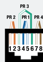
EIA/TIA568B AT&amp;T 258A WIRING
