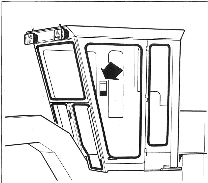
This safety sign is located on the auxilliary switch panel, on the right-hand door post.
