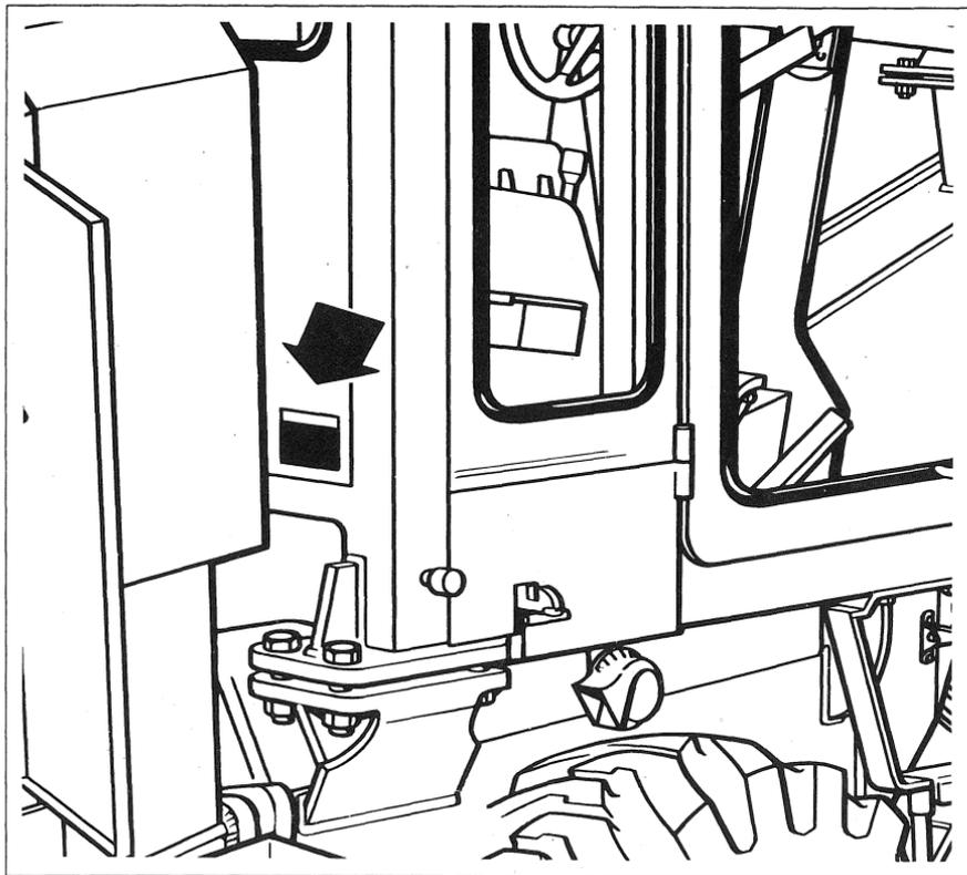
This safety sign is located on the rear right-hand side of the cab.
