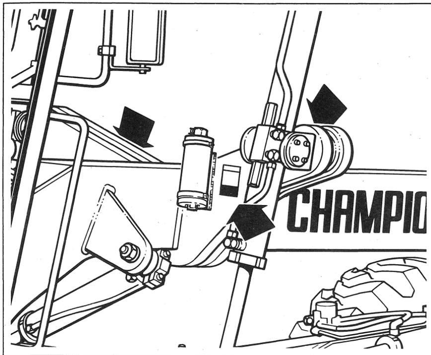
This safety sign appears on or near the accumulator used with blade lift or side shift hydraulic cylinders or oil disc brakes.
